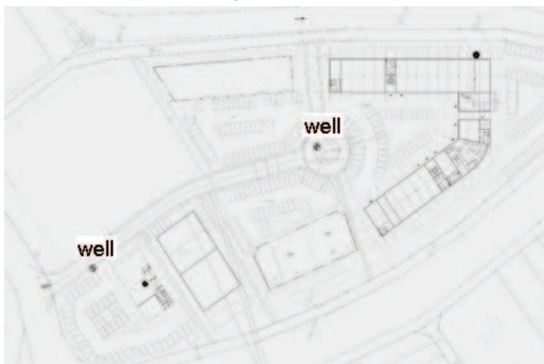
Fig.6.28: Plan of the commercial area in Hainburg to be heated and cooled by GSHP
